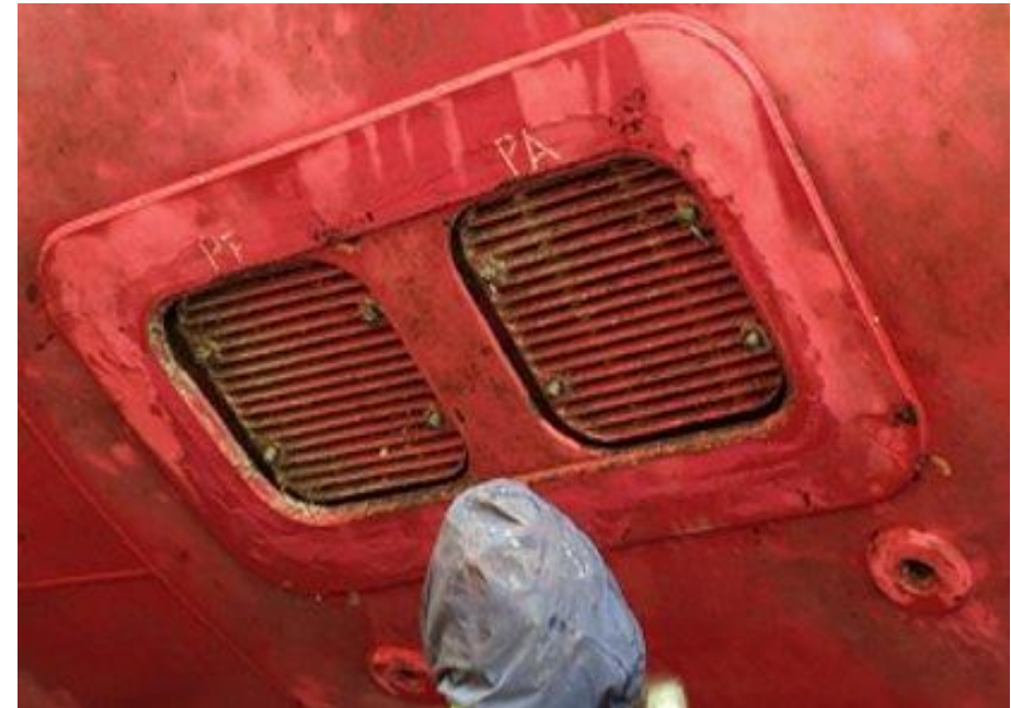
Grating coated with high grade AF of SPC Cu 2 O + Selektope® for coastal LPG carrier (1200DWT) - 16 months
