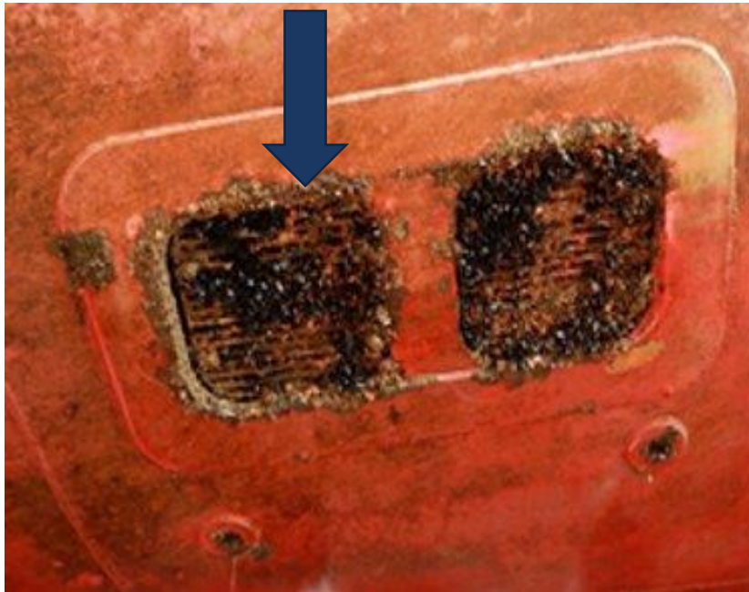
Grating coated with high grade AF of SPC Cu 2 O type for coastal LPG carrier (1200DWT) - 15 months
