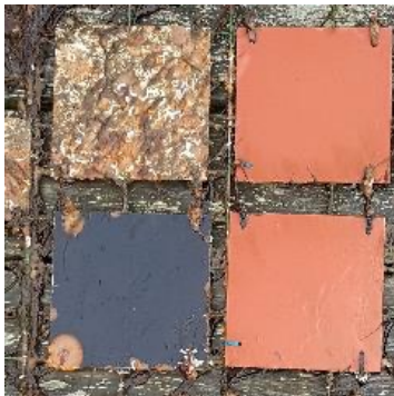
Field testing of coatings
