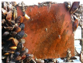
Antifouling biocidal copper coating
