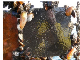
Foul-release biocide-free silicone coating
